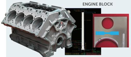
Original casting was failing to meet required tensile properties in the journal bearing area.
