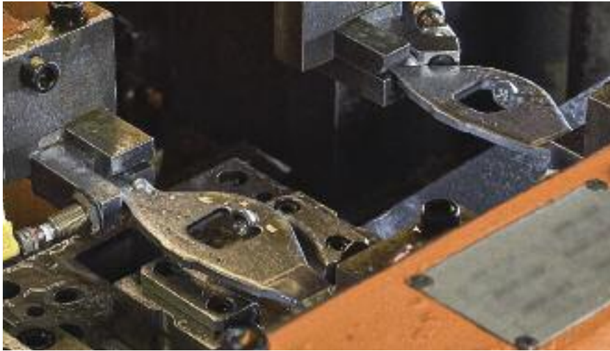
Precision rocker arms move through a high-speed transfer press at Toledo Technologies. A new tool coating has boosted part production and reduced lube use.
