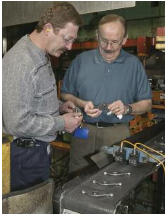
Toledo Technologies' Terry Giesige (left) and Larry Webb examine valve-train components stamped with tooling that employs coatings applied at relatively low temperatures to eliminate distortion, bringing a host of improvements.
