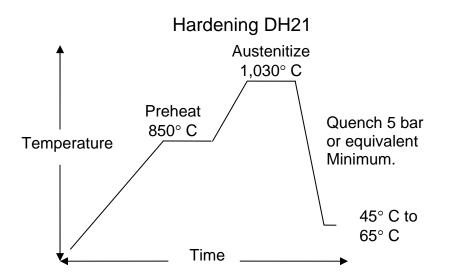
**Vacuum Austenitize & Gas Quenching** – DH21 should first be preheated at a rate of less than 220° C (400° F) per hour and held at 800° C (1,475° F) to 850° C (1,560° F) until the tools are uniformly heated from surface to core to within 60° C (100° F) and then increased to 1,030° C  $\pm 10^{\circ}$  C (1,885° F $\pm 18^{\circ}$  F) to austenitize otherwise known as soaking the tool.
