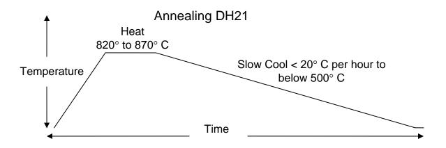
**Annealing** – DH21 can be annealed by uniformly heating the part to between 820° C (1,508° F) and 870° C (1,598° F), and hold for 2 hours followed by a slow cooling at no more than 20° C (36° F) degrees per hour to until the temperature of the part has dropped below 595° C (1,100° F). The part can then be furnace cooled or left in still air to room temperature to complete the annealing process. The part is now ready to be re-hardened.
